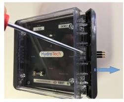
Finish opening the latching mechanism.
