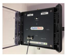
f the fuse is bad, the LED behind the fuse will turn red. Replace the fuse when needed. Fuse type: 20 mm x 5 mm, 1A, 220 V fast blow. Use a small screwdriver to help remove the bad fuse. Insert a new fuse and press down firmly to latch it in place.
