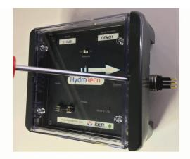
Insert a small flat screwdriver into the small slot on the E-HUB, then push the screwdriver to the right to pry open the latching mechanism.
