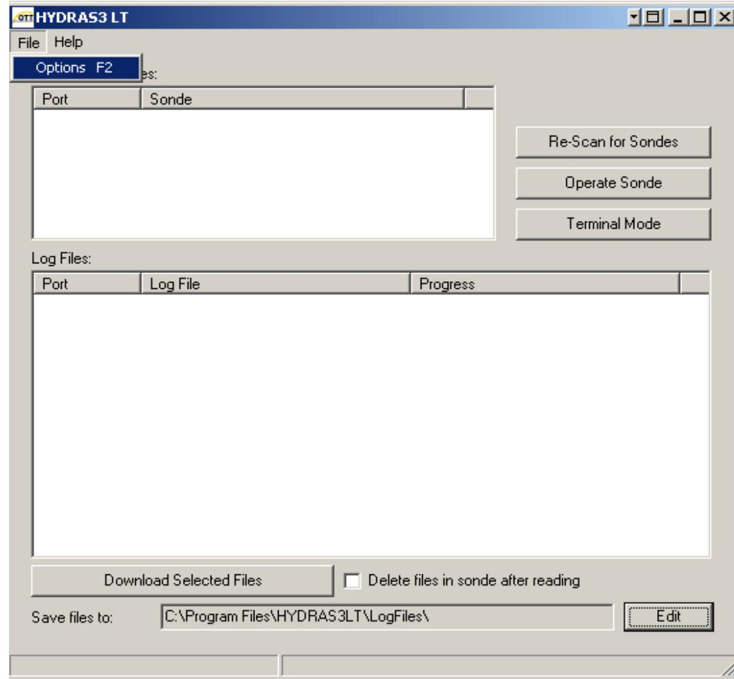
2. If the Sondes/PC baud rate and COM port are known, disable the COM Port and baud rate auto scans and set Hydras3LT to use the known values. This requires Hydras 3LT to concentrate scan activities on only the serial ports of interest.
