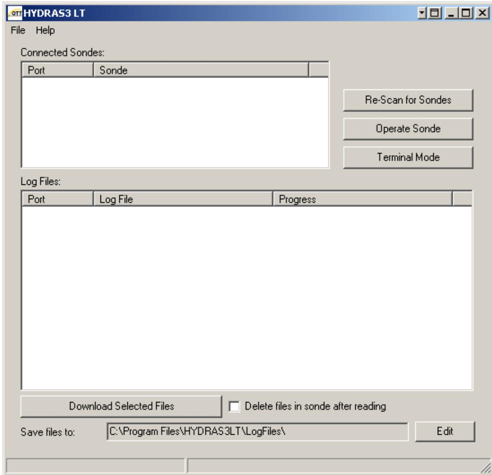
**Note:** For some users with more than one active serial port, it will take some time for Hydras 3LT to try to auto-detect sondes on all ports. It may take up to 30 seconds per active serial port to do the auto-scan.
