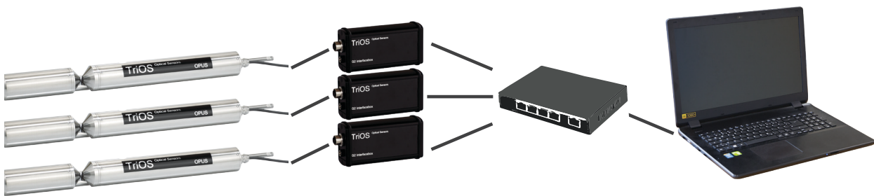
G2 sensors G2 interface box a) Ethernet switch / hub b) Router with DHCP server a) Ethernet-capable device with DHCP server b) Ethernet-capable device
